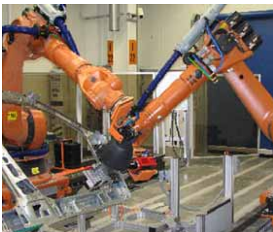
Fig. 4: InfraTec's automated thermographic testing system for non-destructive testing of body panels in the automotive industry
