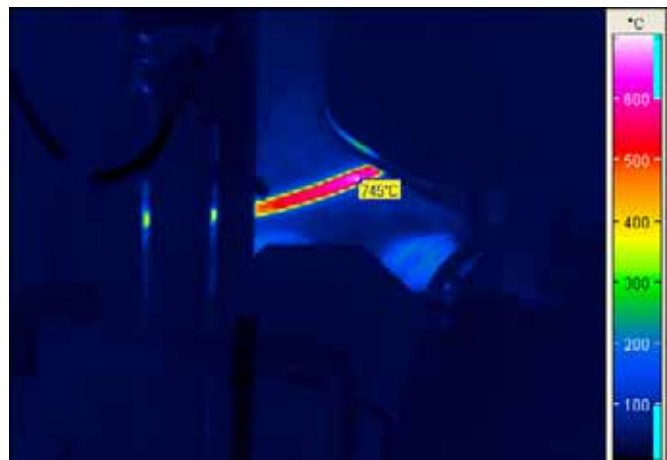
Fig. 3: Thermogram of roller mill for further analysis in a special software
