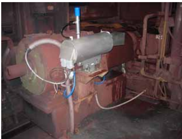
Fig. 2: Automated thermographic measurement system INDU-SCAN for process control – continuous temperature control for sheet metal manufacturing, on-site thermographic camera installation in protective housing with water cooling and air flushing
