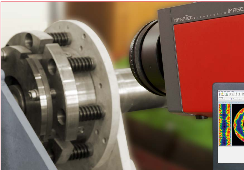
Position of thermal camera in front of the measurement object
